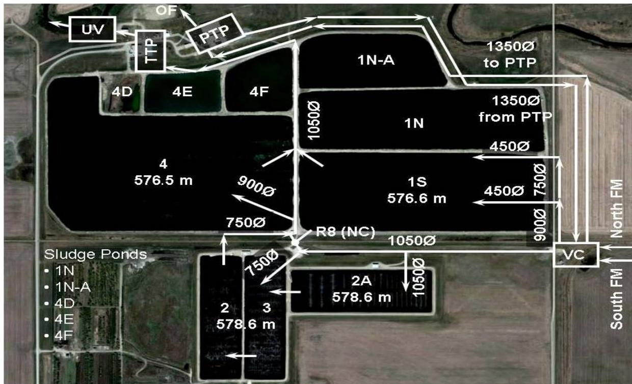
Due to the lack of existing public wastewater infrastructure in the area, the servicing options for the IMF and Industrial Lands Development are generally limited to tying in to either the MBPS forcemains or to the existing valve chamber (VC) located at the southeast corner of the WWTP site.
