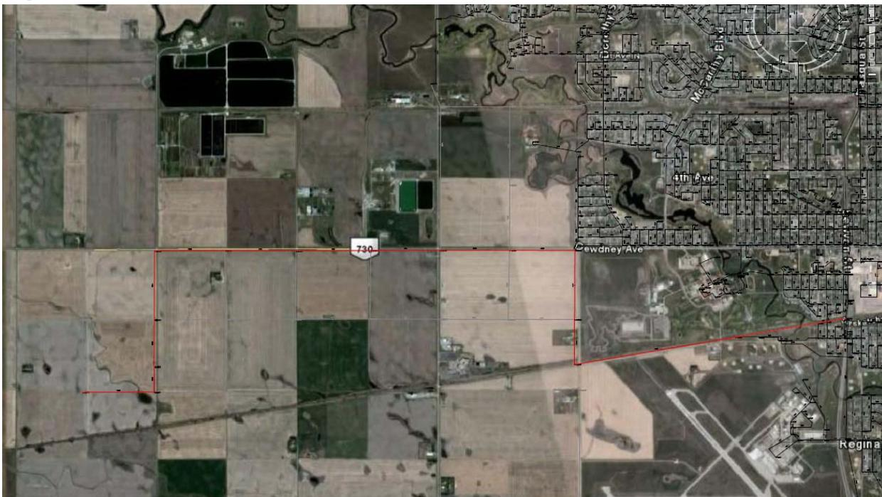
The second alternative would be fed from the nearest existing 300 mm waterline which is located at the intersection of Read Avenue and Toothill Street as shown in Figure 31 – Alternative 2 – Reservoir at Dewdney Avenue and IMF Access. This second alternative, however, was ultimately rejected because it was determined that the existing water distribution system near the western limits of the City could not
