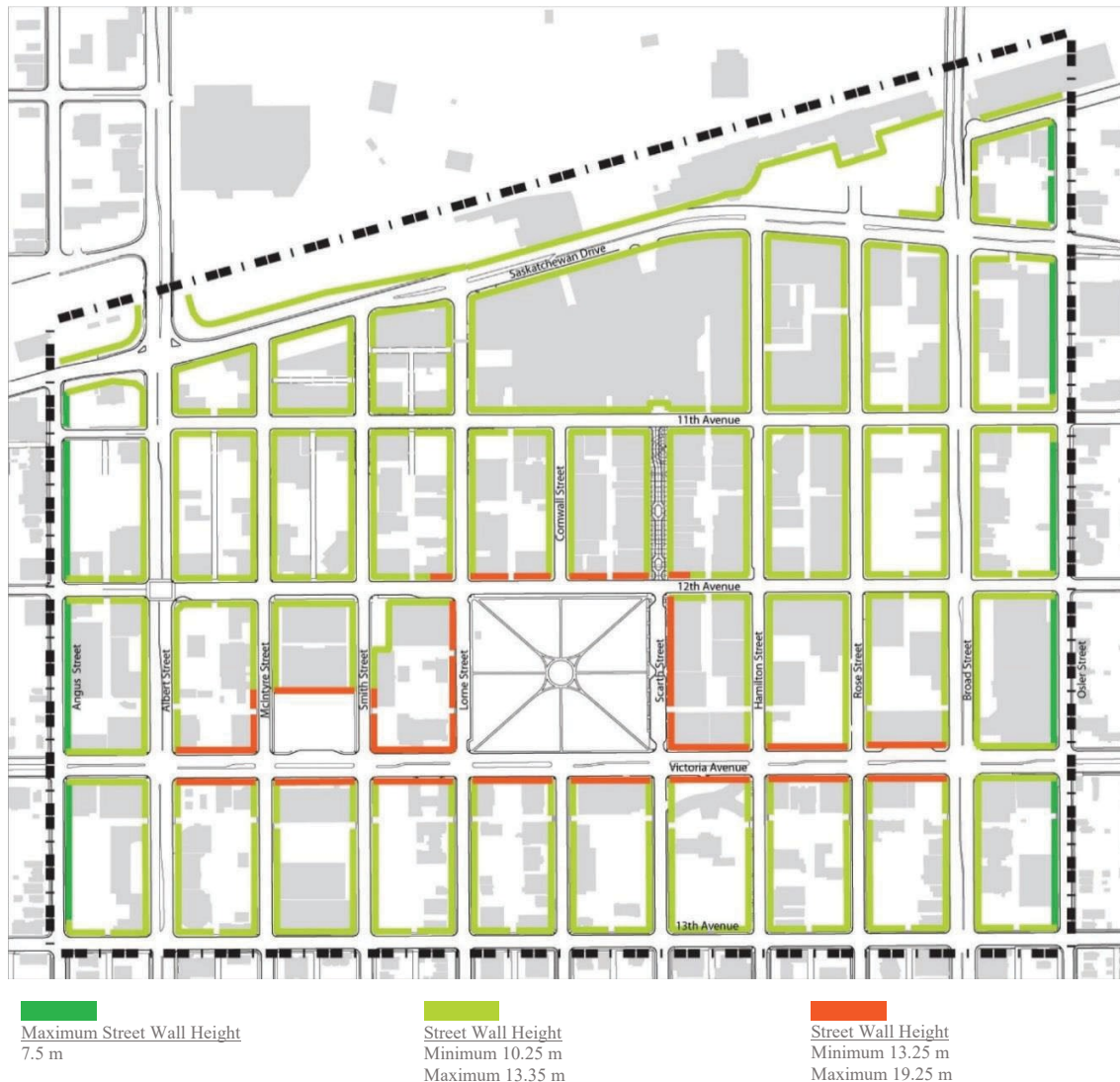
Figure 6A.F4(b): Maximum Street Wall Height
