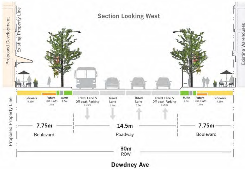
Figure 5-2 Proposed Mid-Block Cross Section
