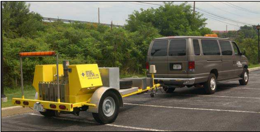
Falling Weight Deflection (FWD) Equipment for Measuring Road Flexibility, i.e. Structural Strength
