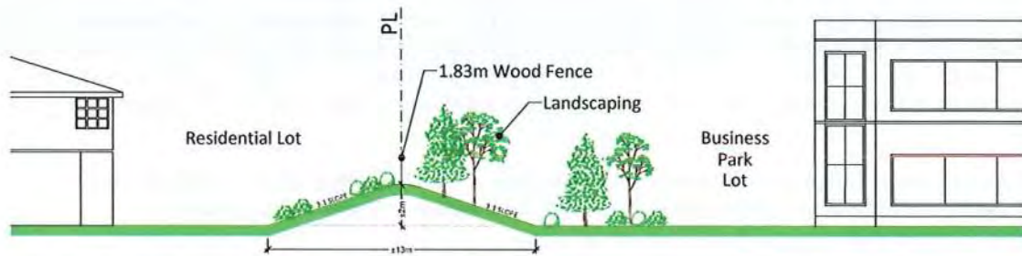
Residential and Business Park Area Interface Treatment Cross Section Scale 1:250
