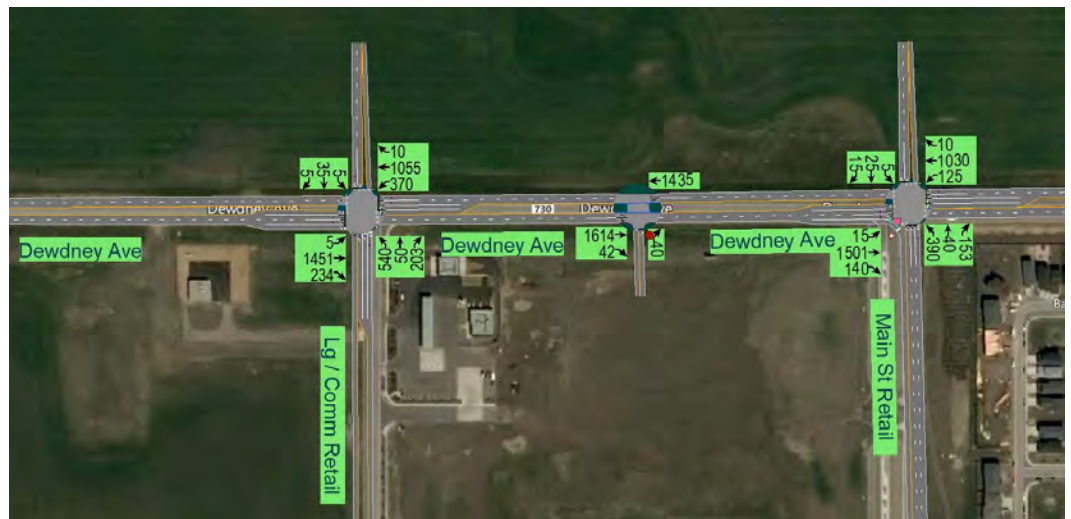
Figure 5 – Driveways traffic with a 10% diversion
