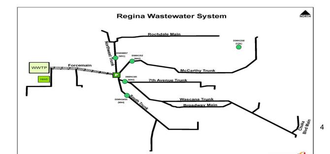
Figure 1. Wastewater Sewer Trunks and Associated Sampling Locations
