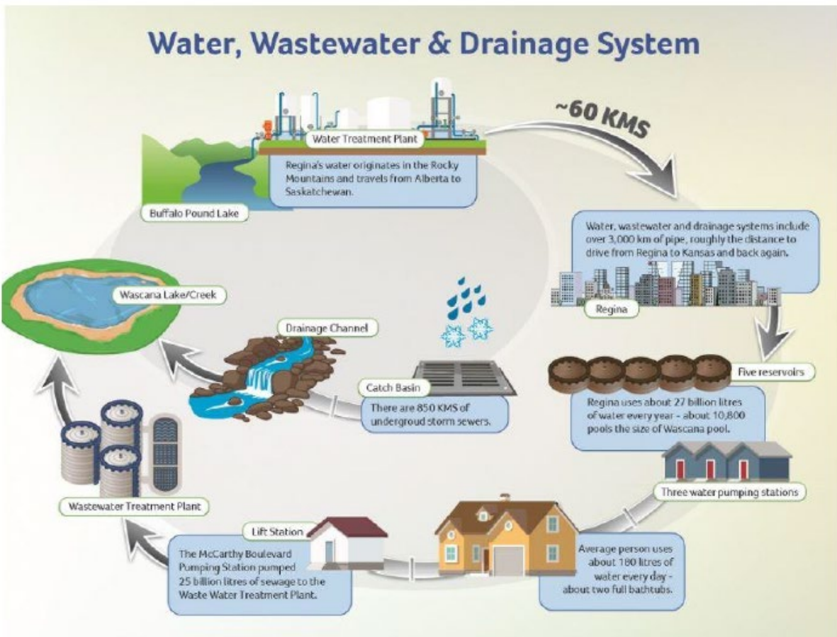
Figure A. Water, Wastewater & Drainage System
